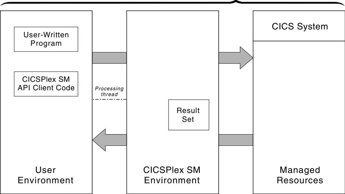
Figure 4. API commands that manipulate managed resources
