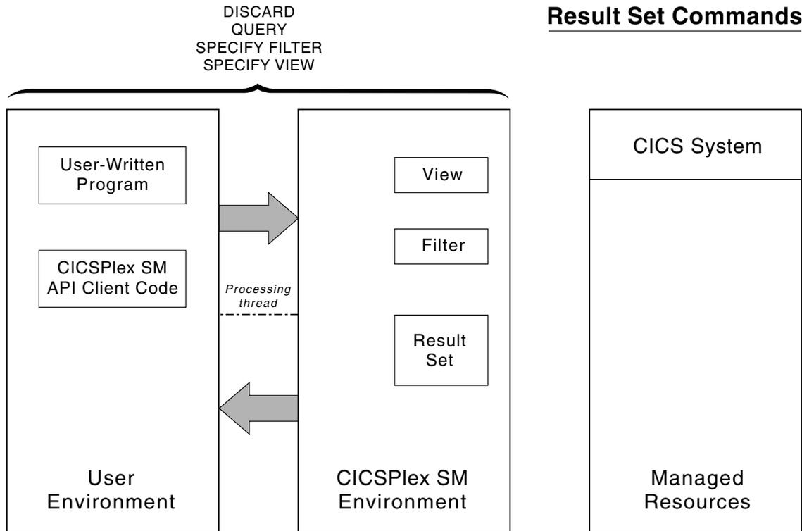
Figure 6. API commands that manipulate result sets
