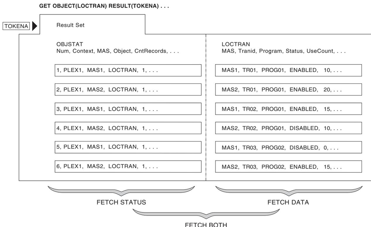
Figure 7. Using FETCH to retrieve result set records
