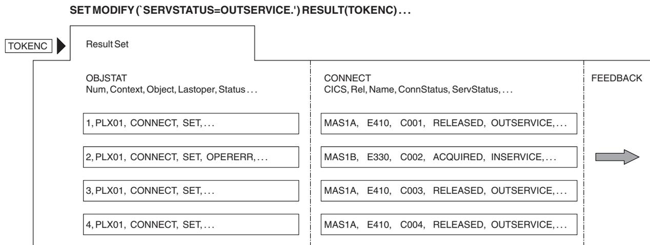
Figure 17. Using SET to modify result set records
