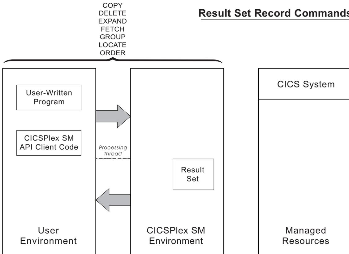
Figure 5. API commands that manipulate result set records
